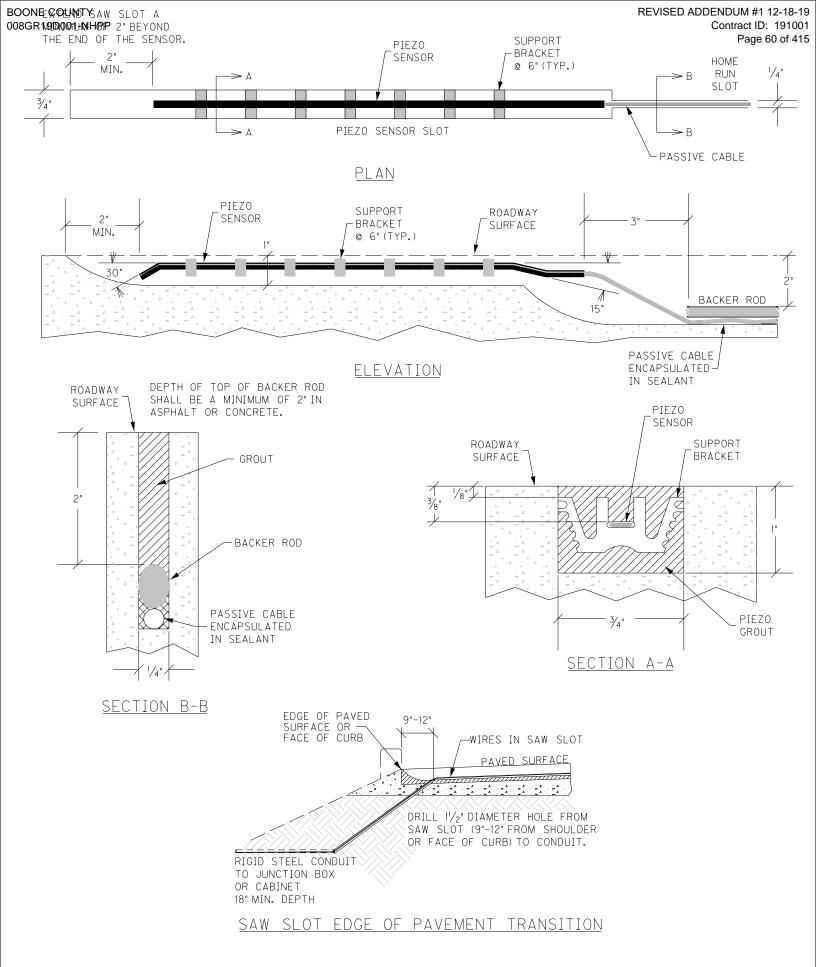
PIEZOELECTRIC SENSOR INSTALLATION
